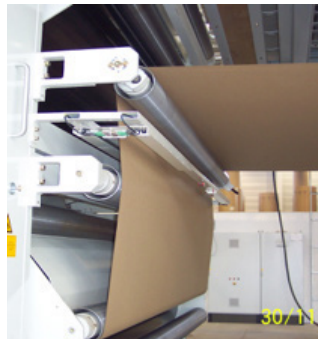
BHS LightGrid Technology for Paper Position Sensing
